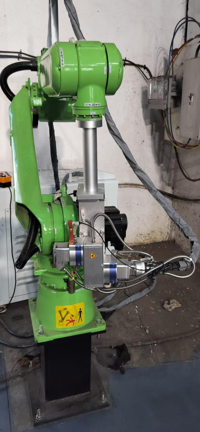
Machine Type: LASER INDUCTION HARDENING MACHINE With Robotic Arm Make: ABB Arm Size- 2.5 Mtr
